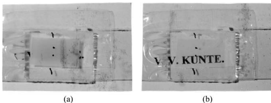
FIGURE 12 Reversible turbid and transparent changes of the PVB/E44 (40/60% w/w) composite film (thickness 12\mu\text{m} ) upon (a) OFF- and (b) -ON under the conditions of 1 KHz AC electric field with 200 V_{p-p} . (See Color Plate VII).
